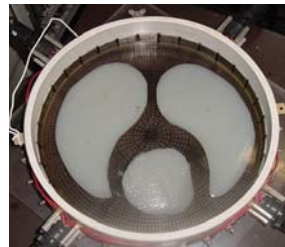
Phantom tank with saline and agar
