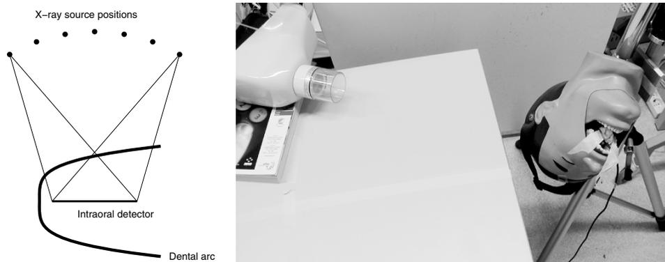
FIG. 5.7. Left: geometry for intraoral measurements. The detector is in fixed position inside the patient's mouth. The source locations are denoted by black dots (7 projections from a total view angle of  $60^\circ$ ). Right: experimental setup.
