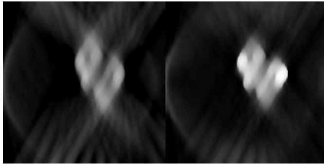
Figure 9. Statistical inference from the posterior distribution for one slice of the tooth data. Nine projections from view-angle of 68^\circ were used as the data. Left: MAP estimate with the (smooth) TV_\beta -prior. Right: CM estimate with the original TV -prior.
