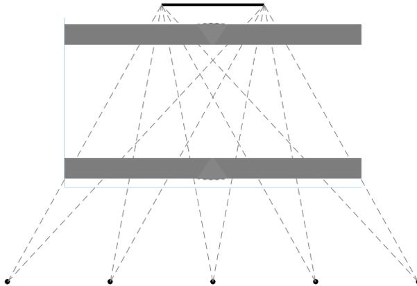
Figure 1: A tomosynthesis type measurement setup using a 10 cm  $\times$  1 cm X-ray detector for the NDT of a 20 mm thick pipe with 150 mm diameter. The pipe has a welded joint in the region of interest close to the detector. The detector is plotted as a thick black line and the source positions are denoted by the black dots. The number of X-ray projections is five, and the total movement of the source is 400 mm.
