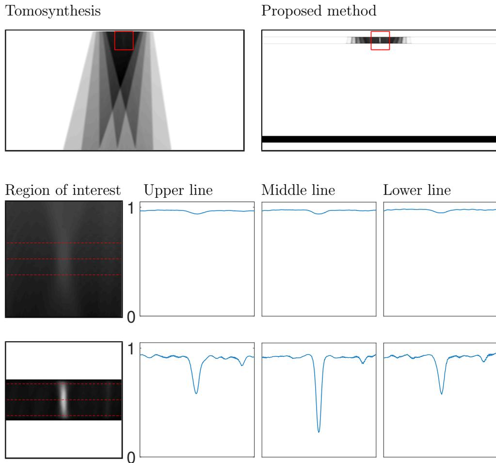
Figure 4: Real data results for an aluminium pipe with a void of 0.5 mm diameter. Top: Reconstructions by tomosynthesis and the proposed TVR-DART variant. Middle row: the region of interest enclosed by the red rectangle in the tomosynthesis reconstruction and the reconstruction profiles on lines indicated by the red dashed lines. Bottom: Same results as in the middle row but for the reconstruction computed by the proposed method.
