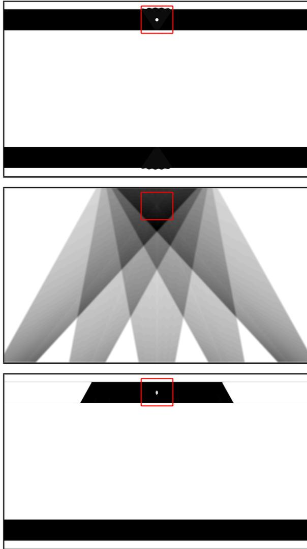
Figure 2: Original phantom (top), tomosynthesis (middle) and the proposed TVR-DART reconstruction (bottom) for simulated data. The areas enclosed by red rectangles are shown in detail in Figure 3. Note that the reconstruction by the proposed method does not precisely follow the shape of the weld; this is due to the fact we assume no accurate a priori knowledge the shape of the weld but use a simple straight-wall approximation.
